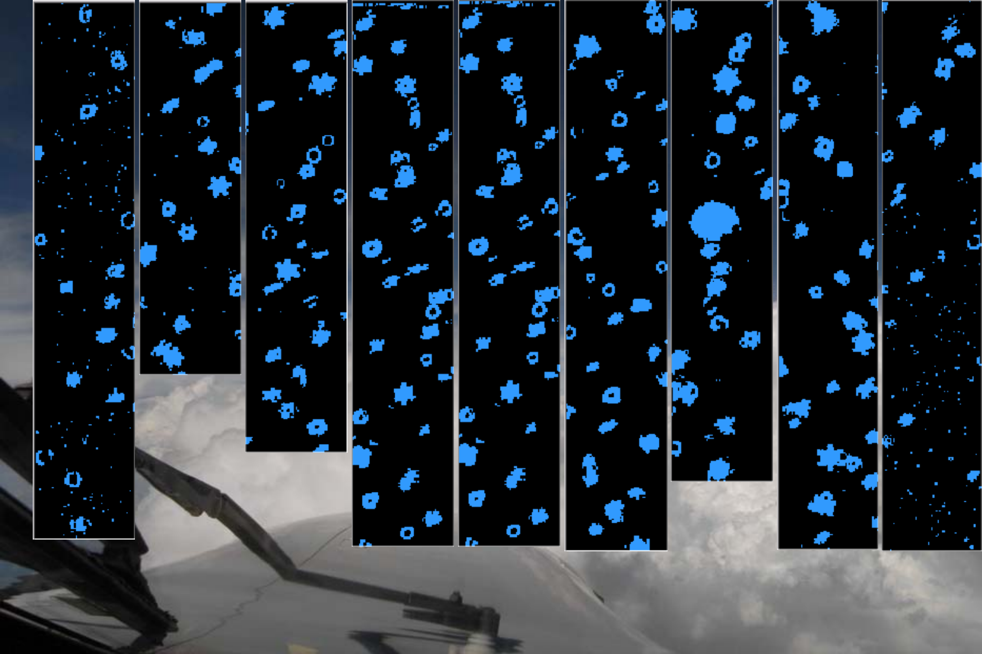
2009 08 24, 9:57 UT, 8130 m, -17.1°C. Max HWLWC=0.49 gm -3 . N of Bareilly. The cloud is glaciating, with frozen rain drops, small graupel and ice crystals.
